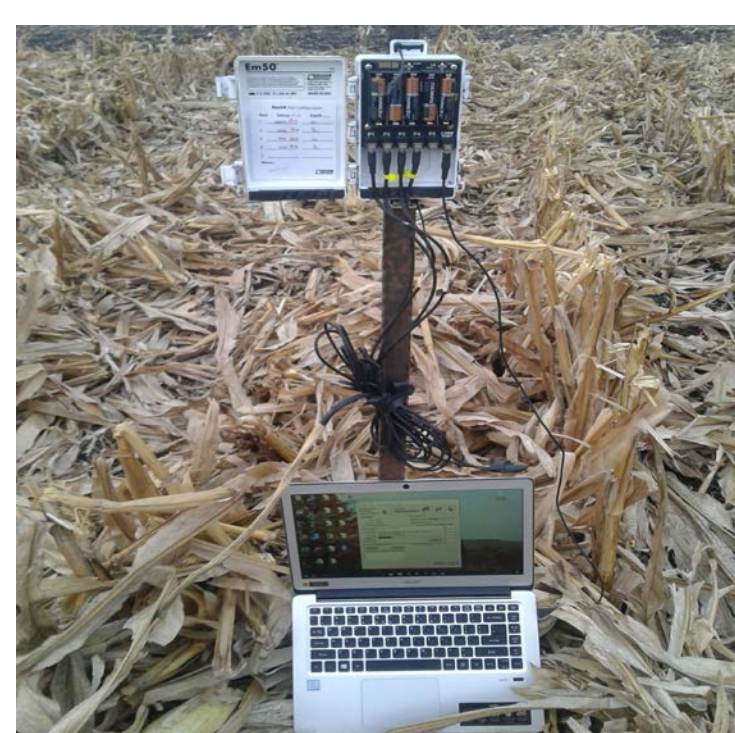
EM50 Datalogger: Downloading soil moisture and temperature data
